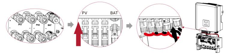
\*\*Note: IN.Hybrid Compact 5.0 M and IN.Hybrid Compact 6.0 M inverter have only two MPPT and two PV strings, so when connecting, you need to unplug ①/② of the PV in the IN.Compact Smartbox.
