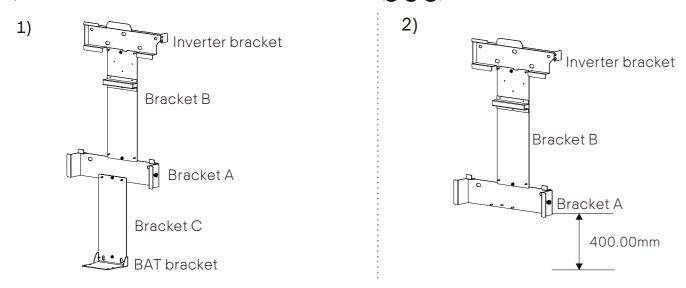
Note: When brackets are mounted, a spirit level is used to keep inverter bracket and Bracket A parallel to the ground.
