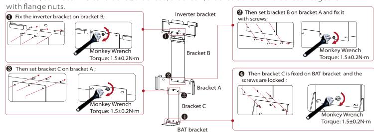
Step 2: Connect the BAT bracket and DZD-BAT SYS-HV-3.0 battery and push the
