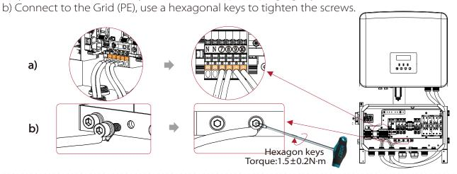
2) PV(PV1+/PV1-/PV2+/PV2-) /Grid(L/N/PE) /Load(L/N) side connection.
