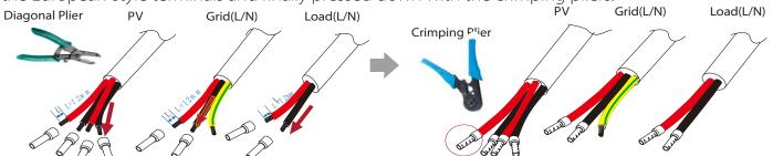
b) Grid(PE) strip the grounding cable, remove the 13 mm insulation layer at the end of the wire.. Insert the stripped cable into the R type terminal, and then clamp it.
