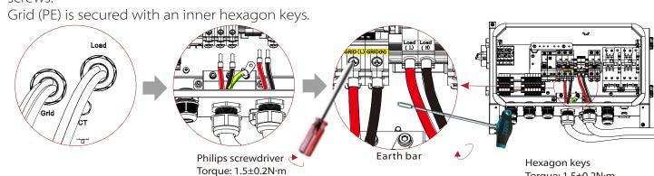
5) Pass the battery power wire through the BAT port of The IN.One Smartbox, then find the BAT+ and BAT-ports in the IN.One Smartbox, insert each wire accordingly, and use the philips screwdriver to lock
