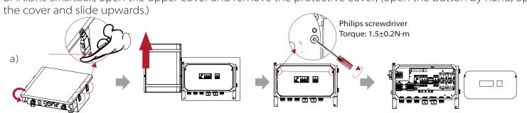
b) Put the IN. One Smartbox on the bracket. Make sure the box is well fixed on the bracket by screwing all
