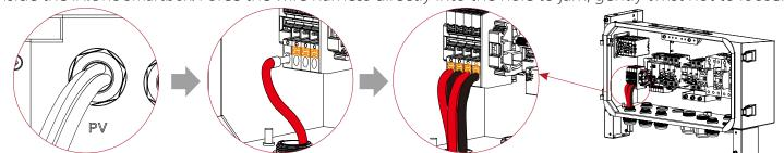
4) Pass the Grid/Load line through the Grid/Load port of the IN.One Smartbox, then find the Grid (L/N) and Load (L/N) ports in the IN.One Smartbox, insert each line accordingly, and use the screwdriver to lock the screws.
